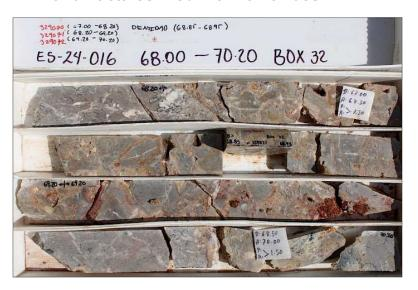
Strong brecciation, calcite recrystallisation and carbonate veining with reddish iron-oxides
